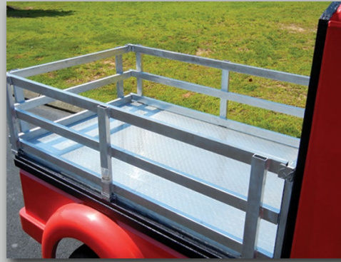
19" high stake backs to hold any equipment
