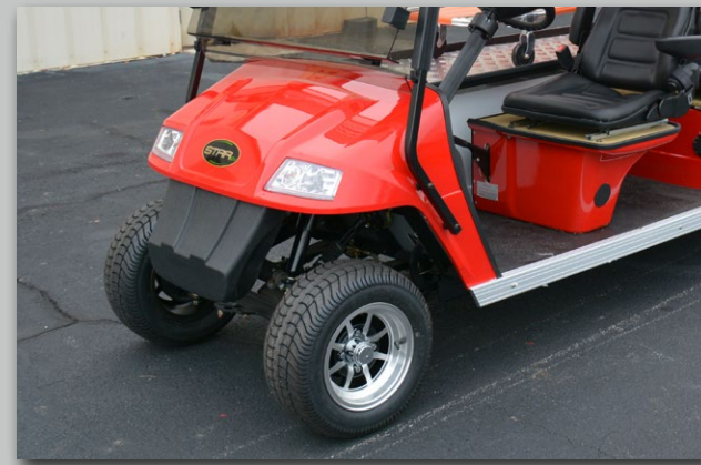
Solid front bumper with rack and pinion steering
