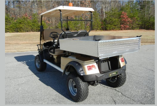
Fold-down tailgate on dumping box
