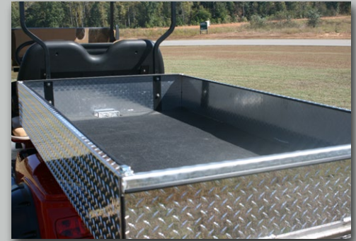
Heavy-duty recycled tire insert
